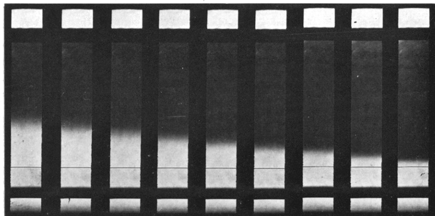
Fig. 2. Sedimentation velocity experiment, followed by absorption at 800 nm, on a purified reaction center from low-iron light particles in 0.1 M potassium phosphate, 0.15% Triton X-100 (w/v), pH 7.5, at 22° ( A_{800 \text{ nm}} = 0.8 ). 59780 rev./min, 8-min intervals.
